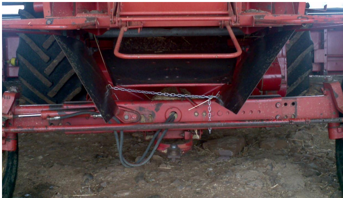
Figure 2 Two pieces of sheet metal arranged to direct the entire trash fraction from the header into a distinct windrow
